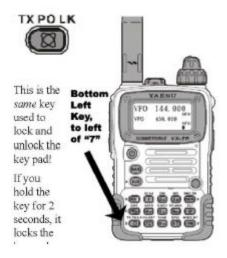
If you hold the key for 2 seconds, it locks the key pad. If you press it just once (or accidentally touch it while holding the radio), it turns wires ON.
